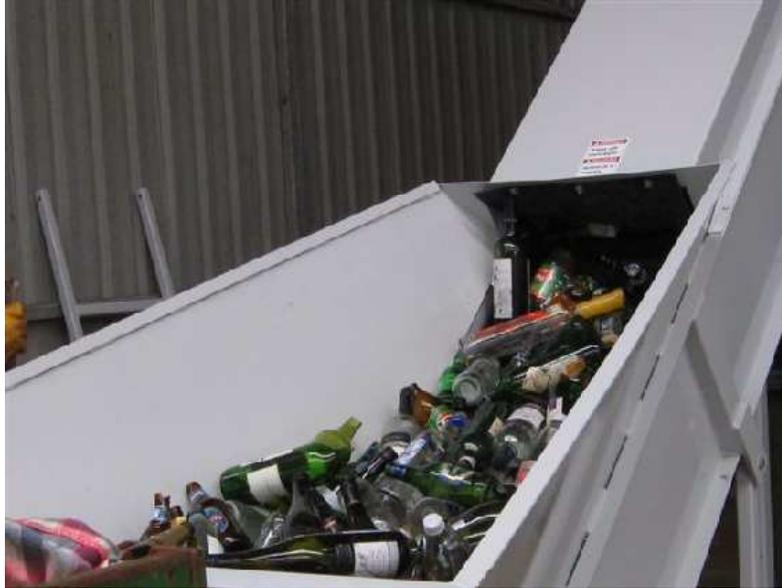
Bottles travelling up the conveyor system into the breaking unit
